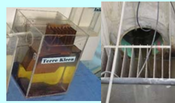
Figure 1. Model and Full-Scale Inclined Plate Settlers: Terre Kleen™ Treatment Device.
